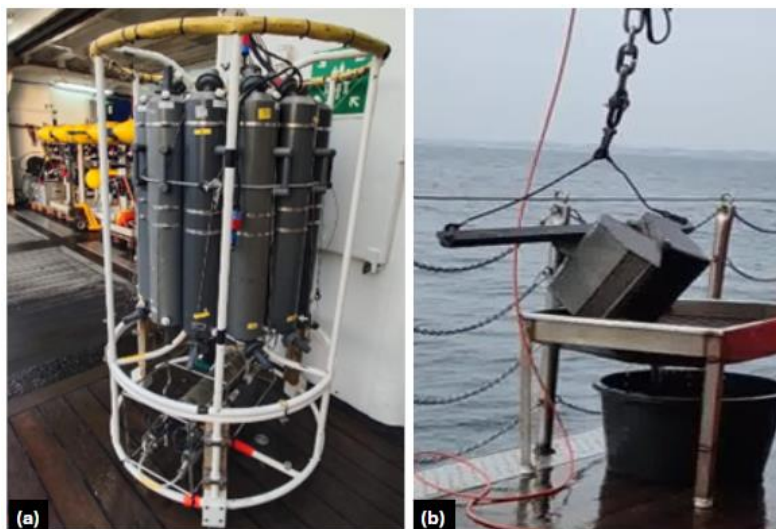
Figure 4: (a) Water Sampler (b) Sediment Sampler
