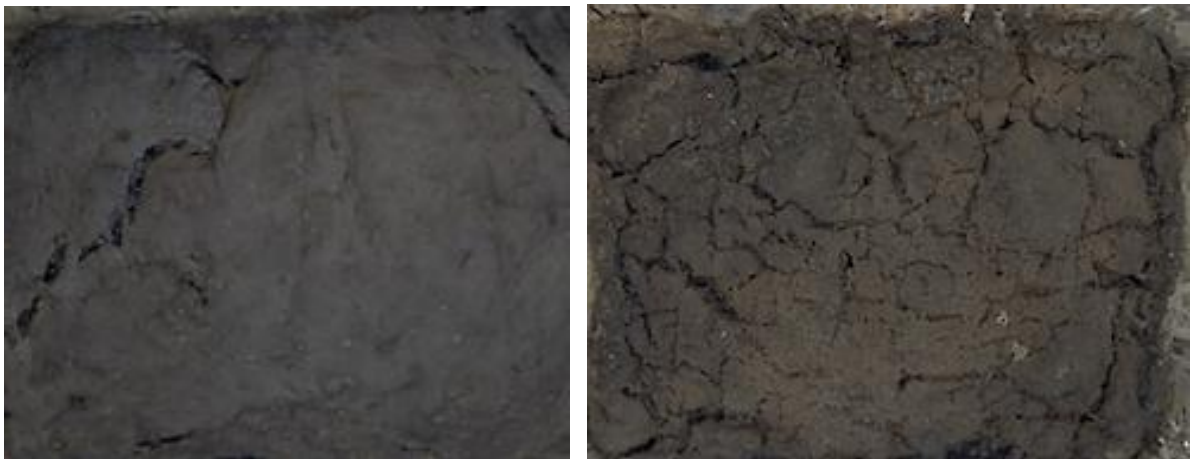
Figure 4-1 The visual comparison of not modified sludge surface (left) and sludge surface modified by SAS application during drying (right).
