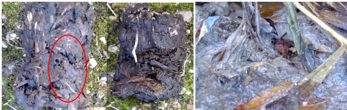
Figure 2-6 Beds development on the first stage bed №2: reed debris in the sludge layer (a), litter accumulation on the bed surface (b).
