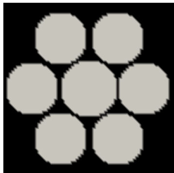
Figure 4.40: Baffle Plate for the Compromise Design
