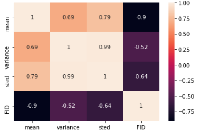
Fig. 5. Pearson correlation matrix between FID, the mean loss value of D, its variance, and its standard deviation. Both FID and the mean loss value are highly inversely correlated.
