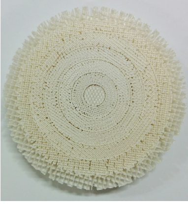
Fig. 4: Three-dimensional printed flat GRIN lens.
