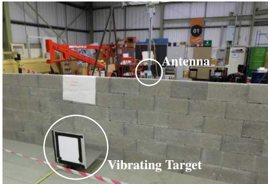
Figure 6: Experimental set-up used for through-wall measurements.
