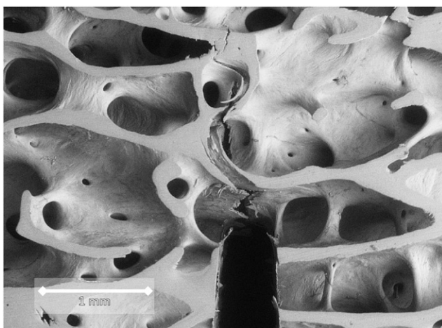
Fig. 1. Crack growth emanating from the man-made notch as in the SENB FT tests of Cook and Zioupos (2009) and Ding and Hvid (2000). Following application of bending moments on either side the notch opens up and the trabeculae ahead of it start snapping. The deformation and crack growth was stopped as soon as this first critical load was reached. The load was used to define the K_{\text{IC}} value (initial notch width \sim 300 \mu\text{m} ).
