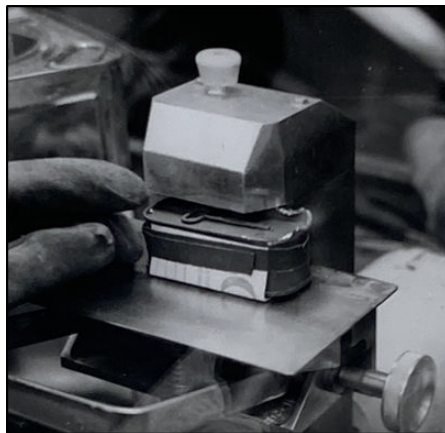
Figure 3. Opening of can using unseaming machine.
