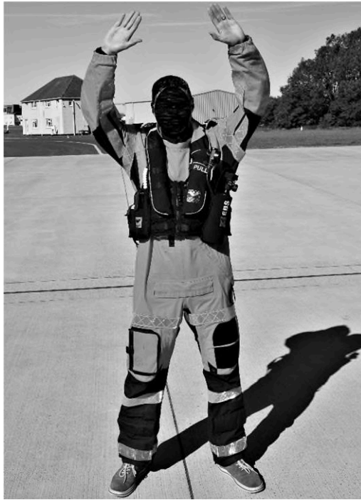
Figure 3 Configuration of retroreflective materials on immersion suit.
