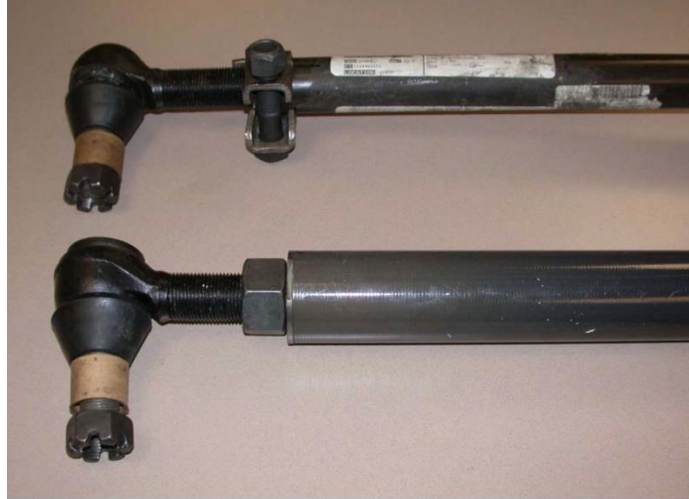
Figure 17: The upper tie rod is a metal tie rod, and the lower one is a CFRP tie rod [15]
