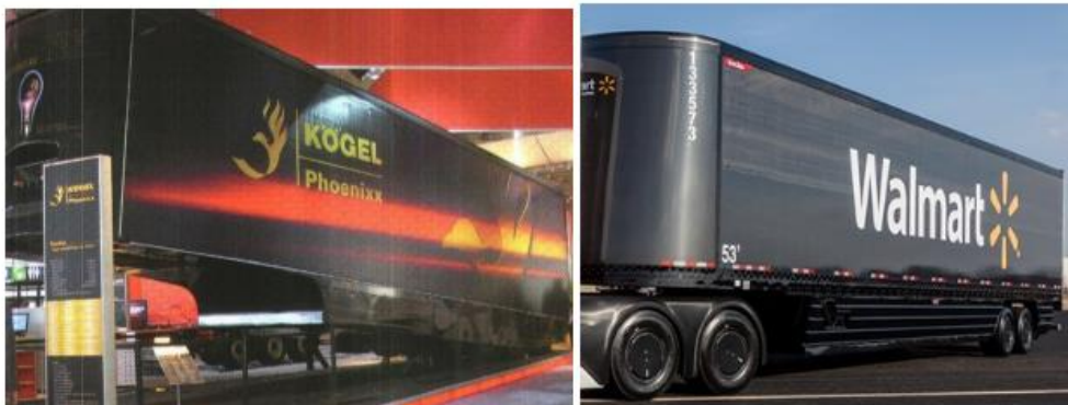
Figure 24: Carbon-fibre epoxy-based composite trailers manufactured by Kögel and Carbotech for Walmart [1]
