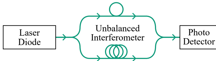
FIGURE 4.1: Example of an unbalanced fibre interferometer in a Mach-Zehnder configuration.
