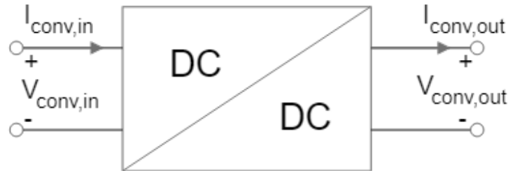
Figure 3.13: A schematic diagram of the low-fidelity DC/DC converter model.
