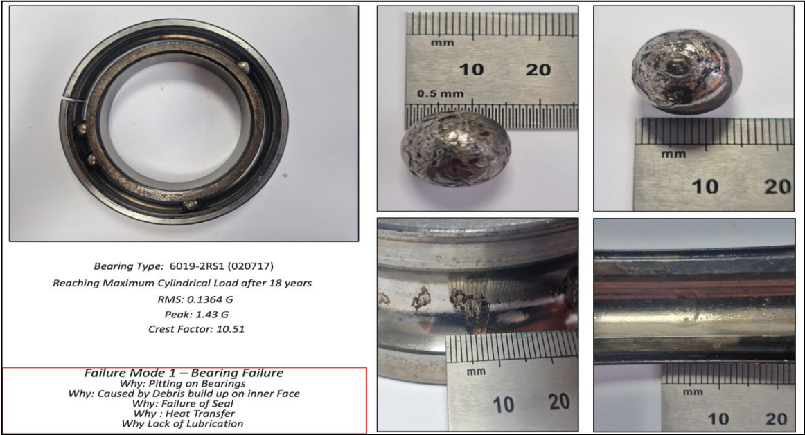
Figure 32 V302 Failure Mode 1
