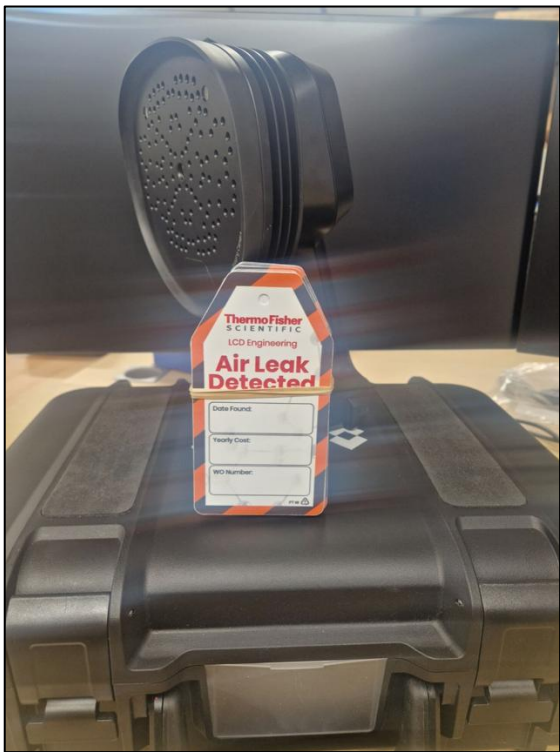
Figure 19 Flir Si-2 and leak detection tags
