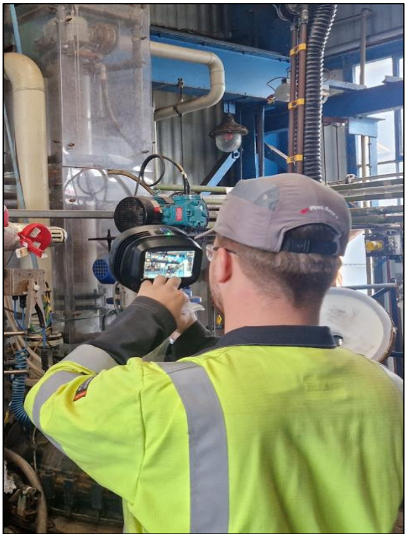
Figure 18 Apprentice at ABC Chemical Manufacturing carrying out AB Ultrasonic Testing
