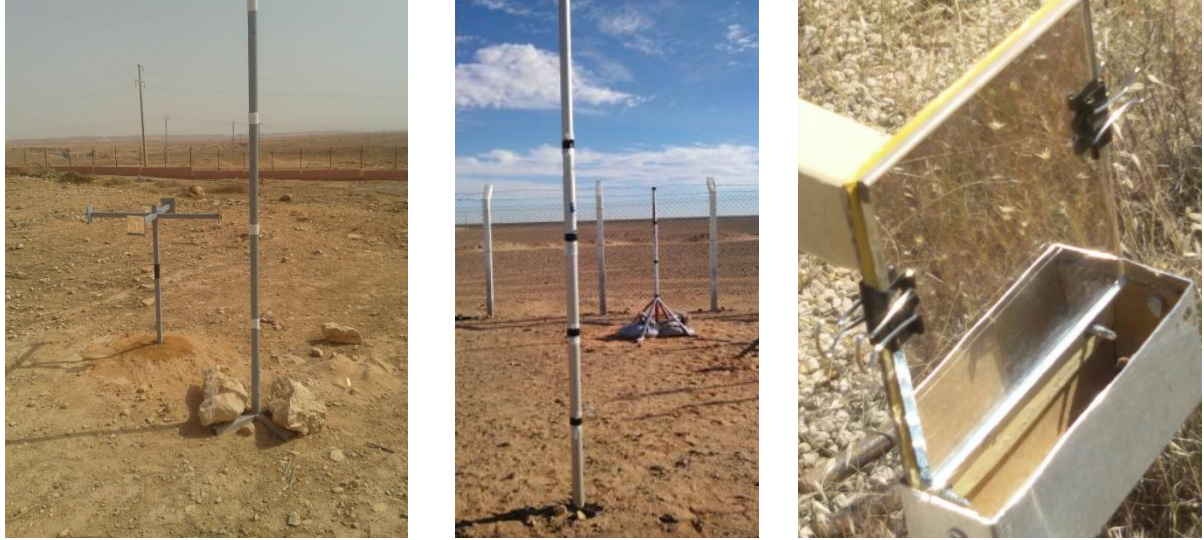
FIGURE 1 (left): Particle collection pole (CDER, Algeria), with glass erosion rig in the background
