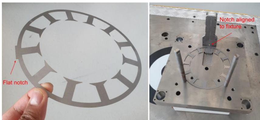
Fig. 15. R3M LamStack Use-Case. [left] Single sheet for the robotic laminated stack application. The sheet is symmetric except for a small flat notch on the outer edge used for alignment. The sheet is flexible, so when held freely, the sheet can be seen to bend in the image. [right] Part of the mounting fixture for the sheet stacking application. The flat notch on the sheet must be aligned to the vertical back plate of the fixture.
