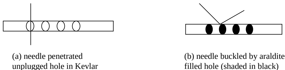
Figure 9. (a) Non-treated and (b) treated Kevlar
