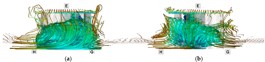
Figure 25. D Streamlines (YZ side view) for a stream velocity of 16.8 m/s for (a) +40; (b) −40 pitch angles.
