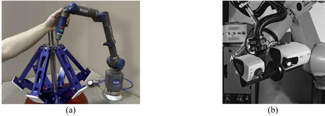
Figure 7. (a). FARO's high-accuracy, 6 axis QuantumS Arm (Technologies, 2018). (b). Fringe projection system mounted on robot end effector (Luhmann, 2010).
