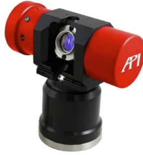
Figure 12. API's active target SMR (API Metrology, 2023).
