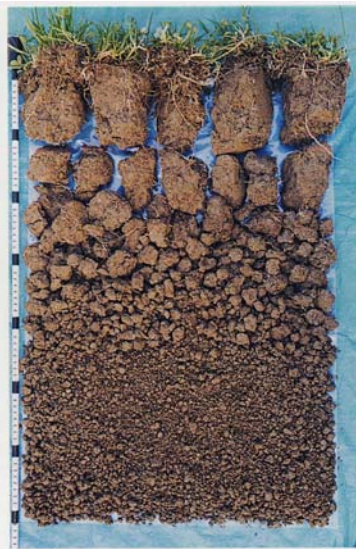
MODERATE CONDITION VS = 1 Soil contains significant proportions of both coarse firm clods and friable, fine aggregates
