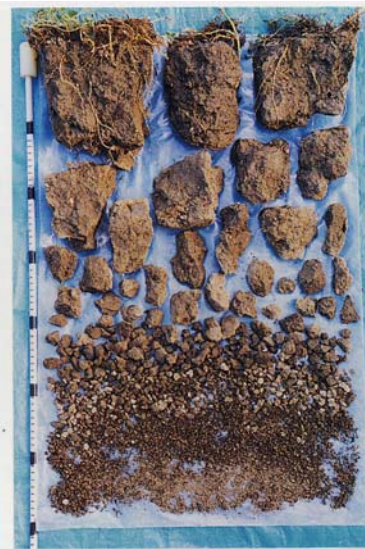
POOR CONDITION VS = 0 Soil dominated by extremely coarse, very firm clods with very few finer aggregates
