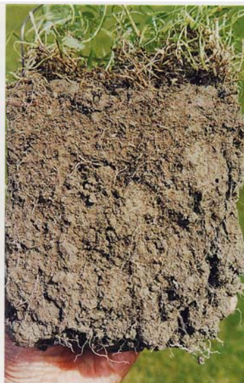
MODERATE CONDITION VS = 1 Soil macropores between and within aggregates have declined significantly but are present on close examination of clods showing a moderate amount of consolidation
