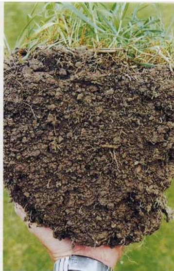
GOOD CONDITION VS = 2 Soils have many macropores between and within aggregates associated with readily apparent good soil structure
