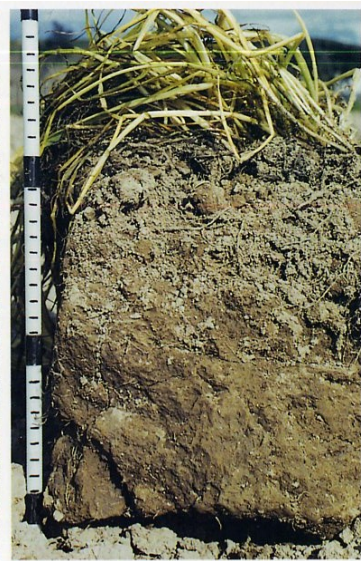
POOR CONDITION VS = 0 Very firm to hard, well-developed tillage pan in the lower topsoil, showing severe consolidation with no structure, no macropores and few or no cracks
