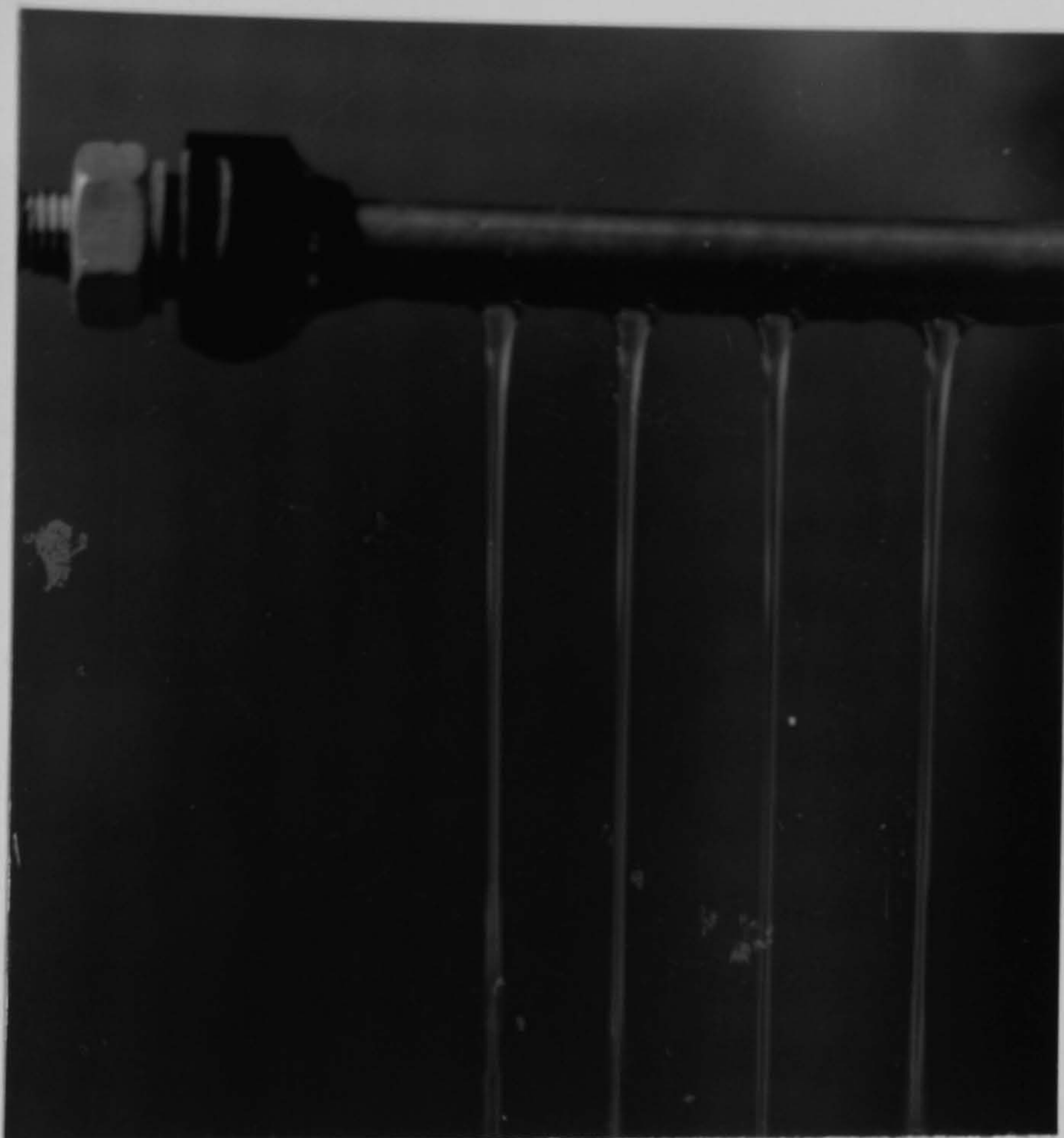
Figure 4.5a The feed system of the Micron X-15 emitting Glossinex at 0.2 litres/minute
