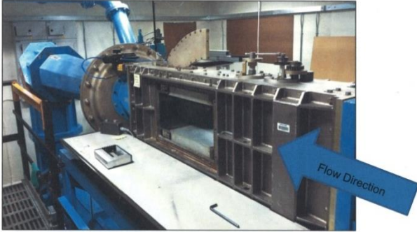
Figure 2. Transonic wind tunnel with side door removed
