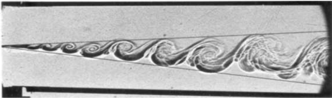
Figure 1.7: Example of the shadowgraphs of a plane-mixing layer (Brown & Roshko, 1971).
