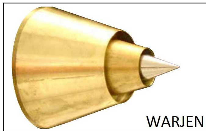
Figure 6.2: The short cowl coaxial nozzle (WARJEN) from the experiment of (Eastwood et al. , 2008).
