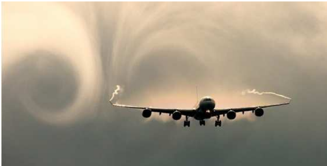
Figure 1.5: Picture of the trailing vortices of a civil airliner during landing. (Online, 2011).
