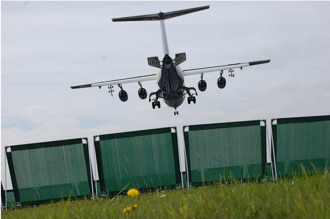
Figure 1.20: FAAMs BAe 146-301 Atmospheric Research Aircraft in field trials at Cranfield University and the tested baffle array (final baffle design) (Bennett et al. , 2013).
