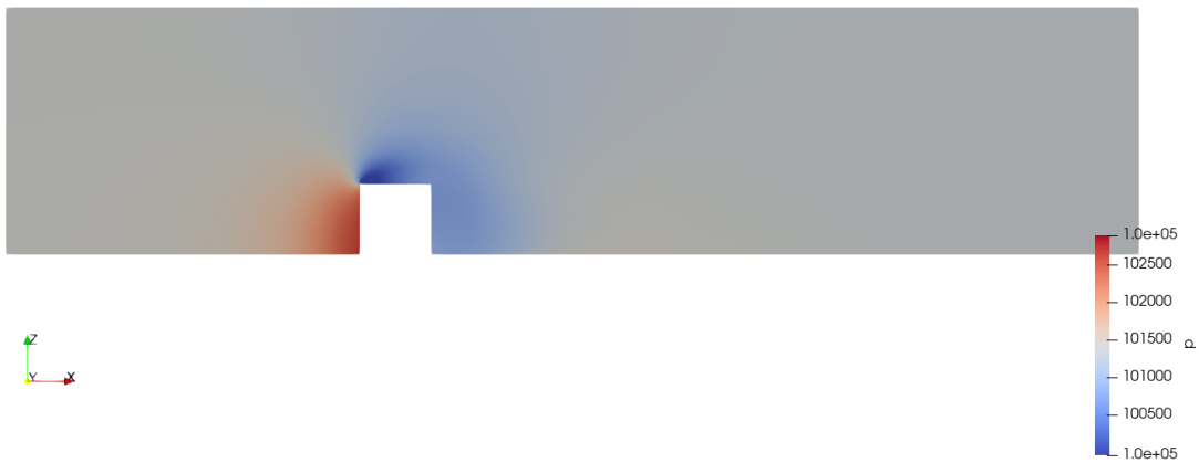
Figure 4.19: Pressure distribution on the side face ( x -constant plane) at t = 20 s.
