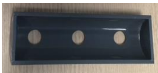
Figure 4.1 Prototype of 150 mm acrylic sampling tube containing 2 x end baffles (250 mm depth) and 3 x 15 mm drainage holes. At an up-scaled size, for the monitoring project, 4 lengths of 0.5 m were joined together with resin to form a 2 m length that would be placed across the whole cage width when filling with sewage sludge cake.
