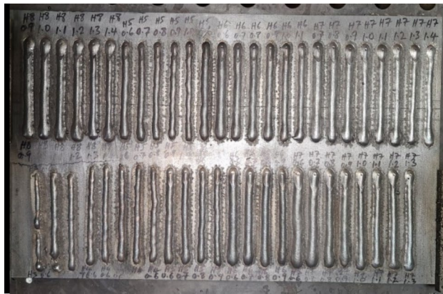
Fig. 8 Bead-on-plate for process selection using S355 baseplate
