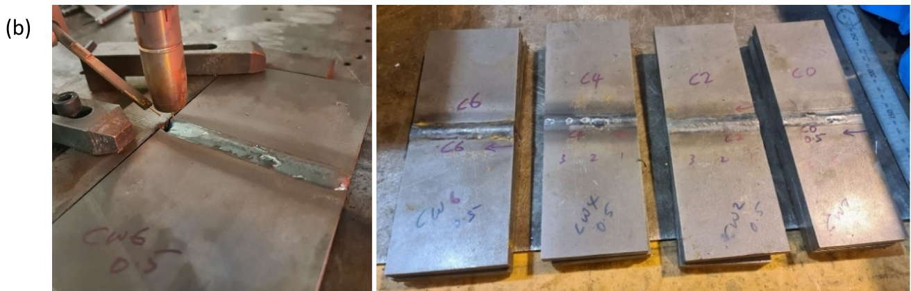
Fig. 13 a Schematic of butt joint; b welded plates for tensile samples' extraction
