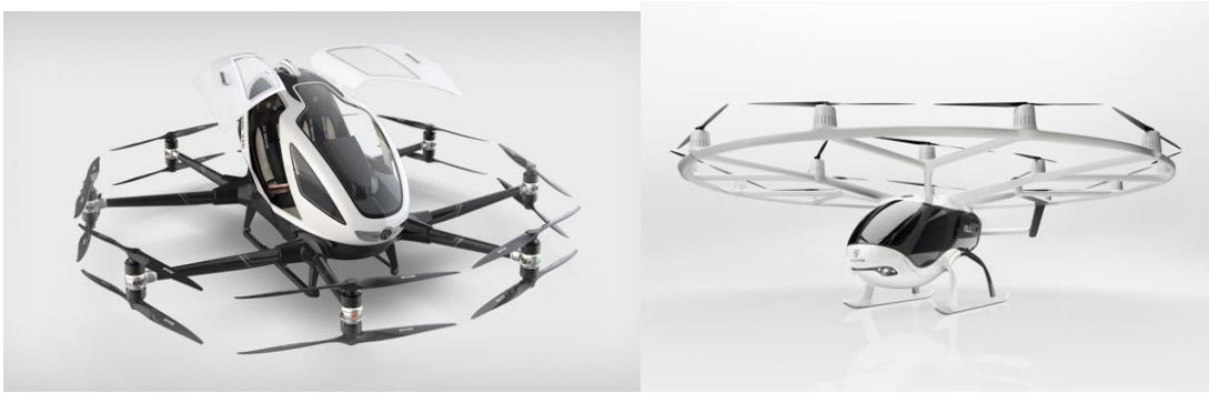
Figure 2-4 Wingless eVTOLs: EHang 216[4]; VoloCity 2X [7]
