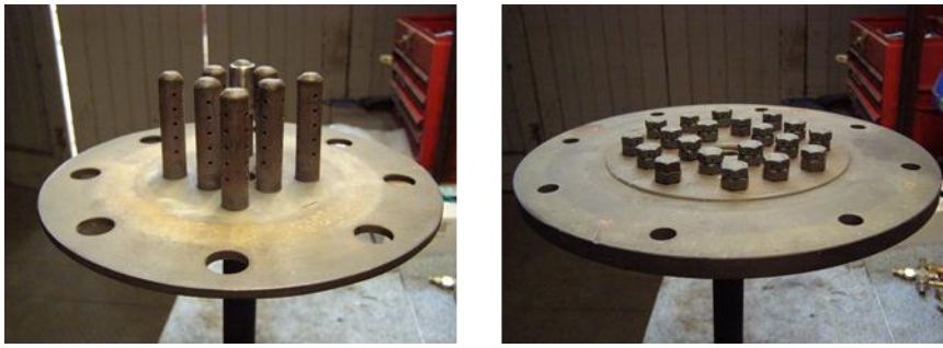
Figure 6-4 a) Carbonator gas distributor comprising eight nozzles; b) Calciner gas distributor comprising twenty nozzles.
