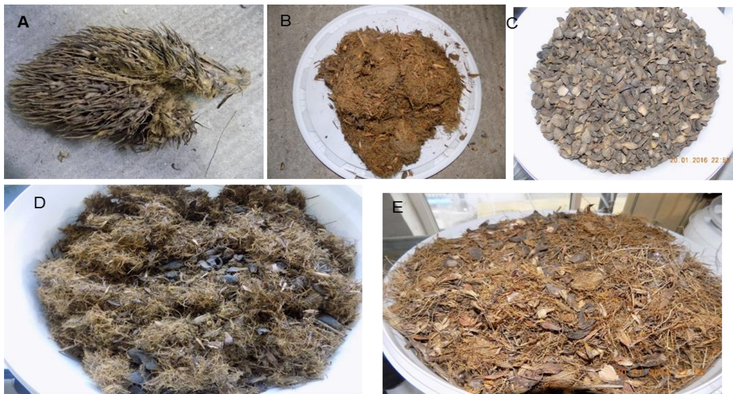
Figure 5-3 Fresh fruit bunch solid wastes (A) empty fruit bunch, (B) mesocarp fibre, (C) palm kernel shell, (D) mixture of empty fruit bunch, mesocarp fibre, and palm kernel shell of 0.0067 m particle size, and (E) mixture of empty fruit bunch, mesocarp fibre, and palm kernel shell of 0.0140 m particle size.
