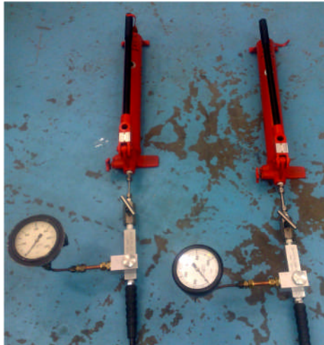
Figure 4-9 Hydraulic pump and pressure gauge installed on the test rig
