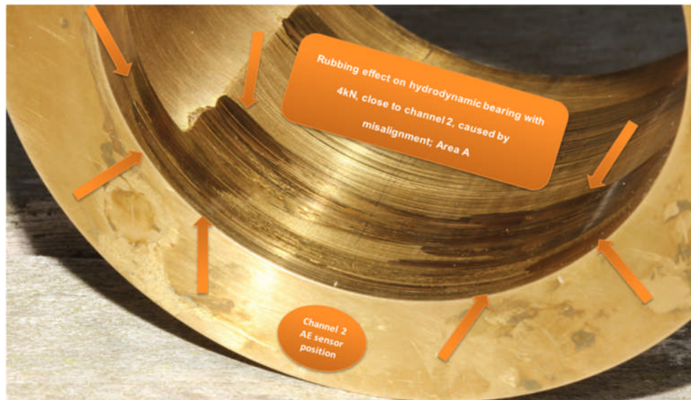
Figure: 7-12 Influence of rubbing on hydrodynamic bearing close to channel 2
