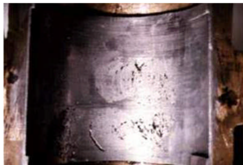
Figure 2-11 Initial Deterioration (Neale Consulting Engineers)
