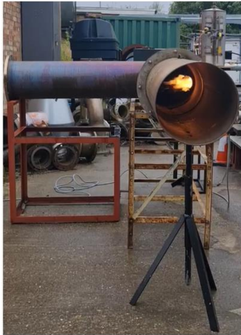
Figure A-9: Burner system being tested.
