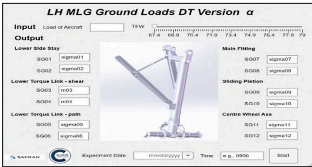
Fig. 5. MLG ground loads (force and torque) DT version \alpha interface
