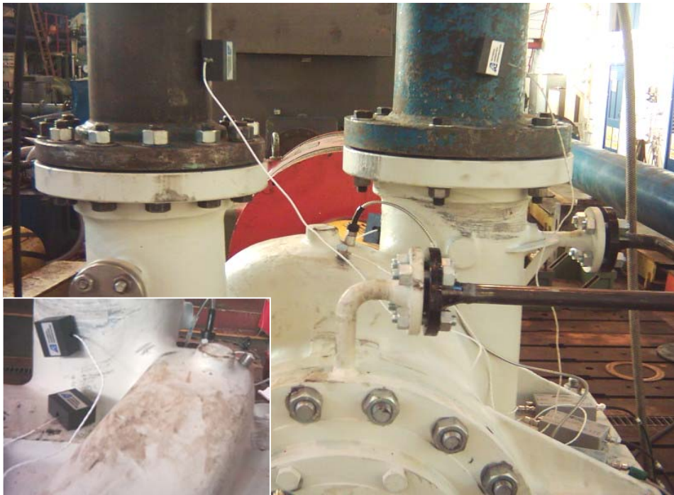
Figure 1 60KW centrifugal pump which underwent performance and NPSH tests showing AE sensor locations
