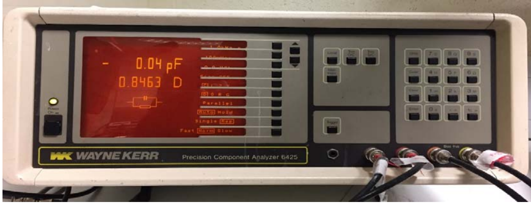
Figure 2-12: Photo to the device that used to measure the dielectric properties at room temperature and at different frequencies.
