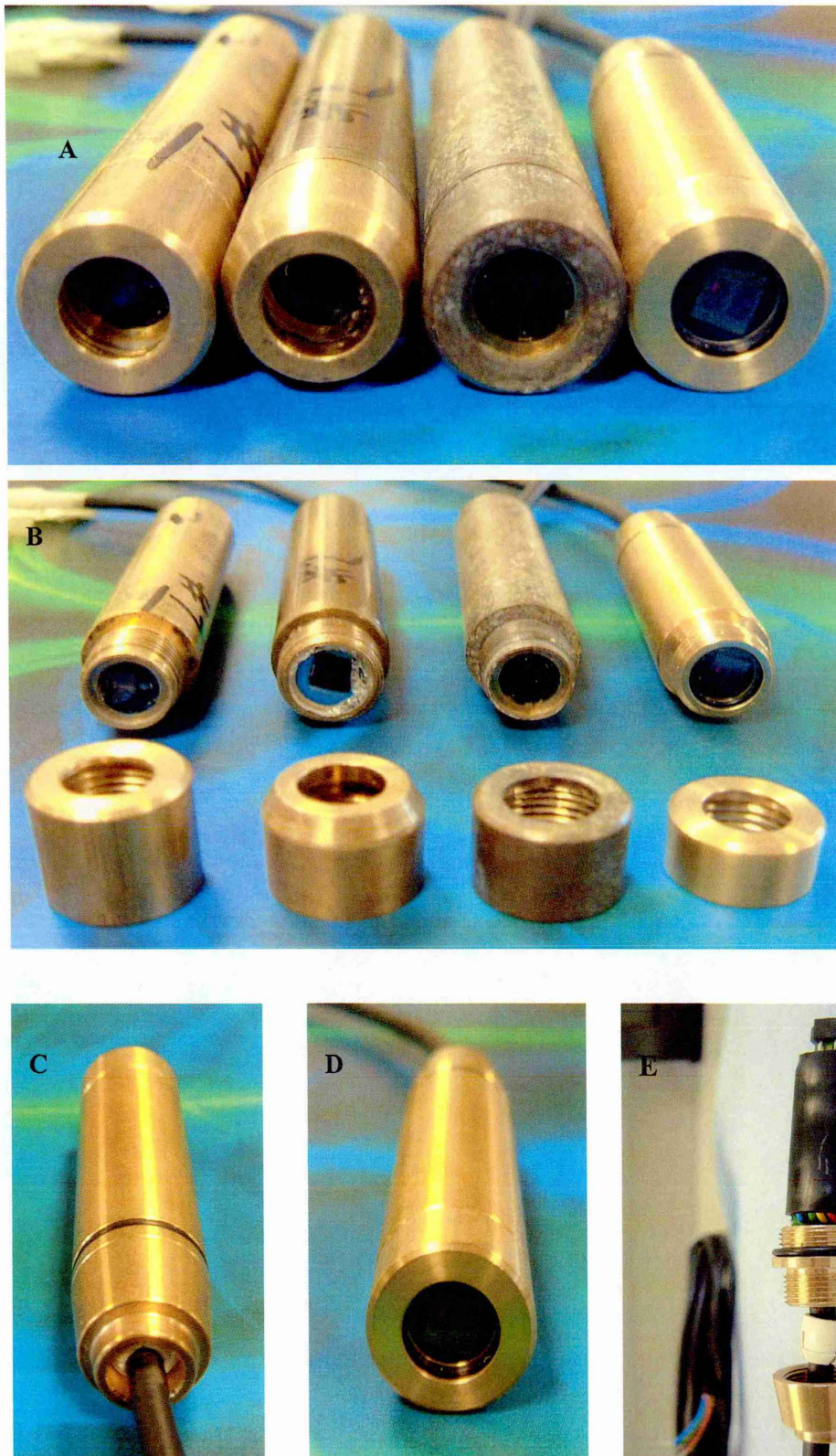
Fig. 2.9 The development of the Mk1 sub-surface fuel sensor to the superior Mk 4 design. A) Assembled sensors Mk 1-4 (left to right) showing decreasing head recesses; B) Mk 1-4 sensors showing sequential reduction of head length and minimised front recesses. The protective glass lip on the Mk 4 sensor is evident; C) Mk 4 sensor (rear); D) Mk 4 sensor with head assembled (face front); E) Sealed internal components of the Mk 4 sensor and reinforced cable exit assembly. The NIR unit is shown top. The reinforced cable exit (bottom) is shown dismantled.
