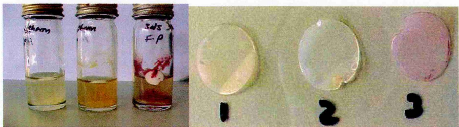
Fig. 4.30 Membrane post-inoculation with the crop fungus F. poae . Extensive growth on one replicate is shown (left). All 3 membranes turned translucent on exposure to diesel (8 \mu l) regardless of the degree of colonisation or discoloration (as seen right - 3).
