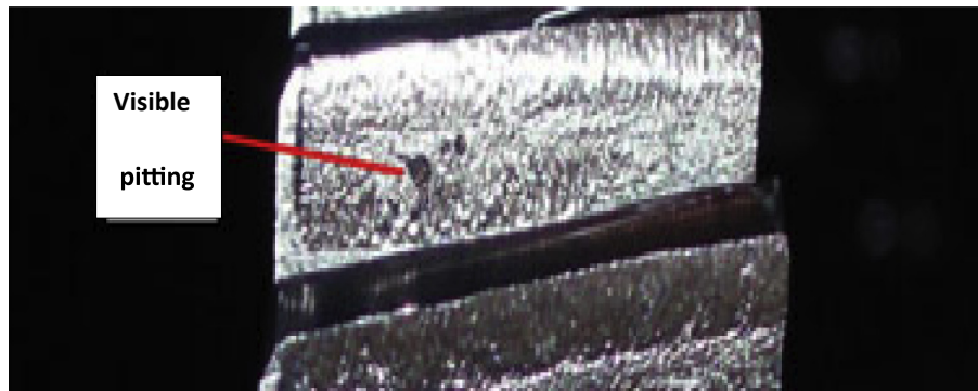
Fig. 12. Visible pitting after test 1 [50].
