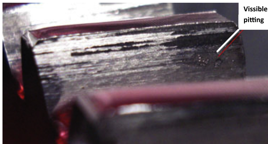
Fig. 13. Visible damage after test 2 [50].
