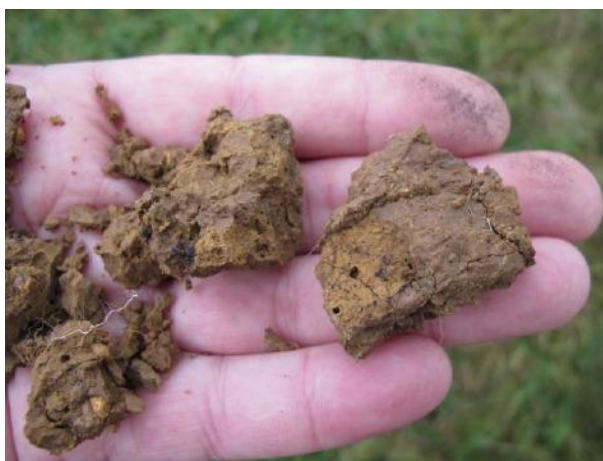
Figure 3 Slickensides, or clay shear plates. ( S. Hallett )
