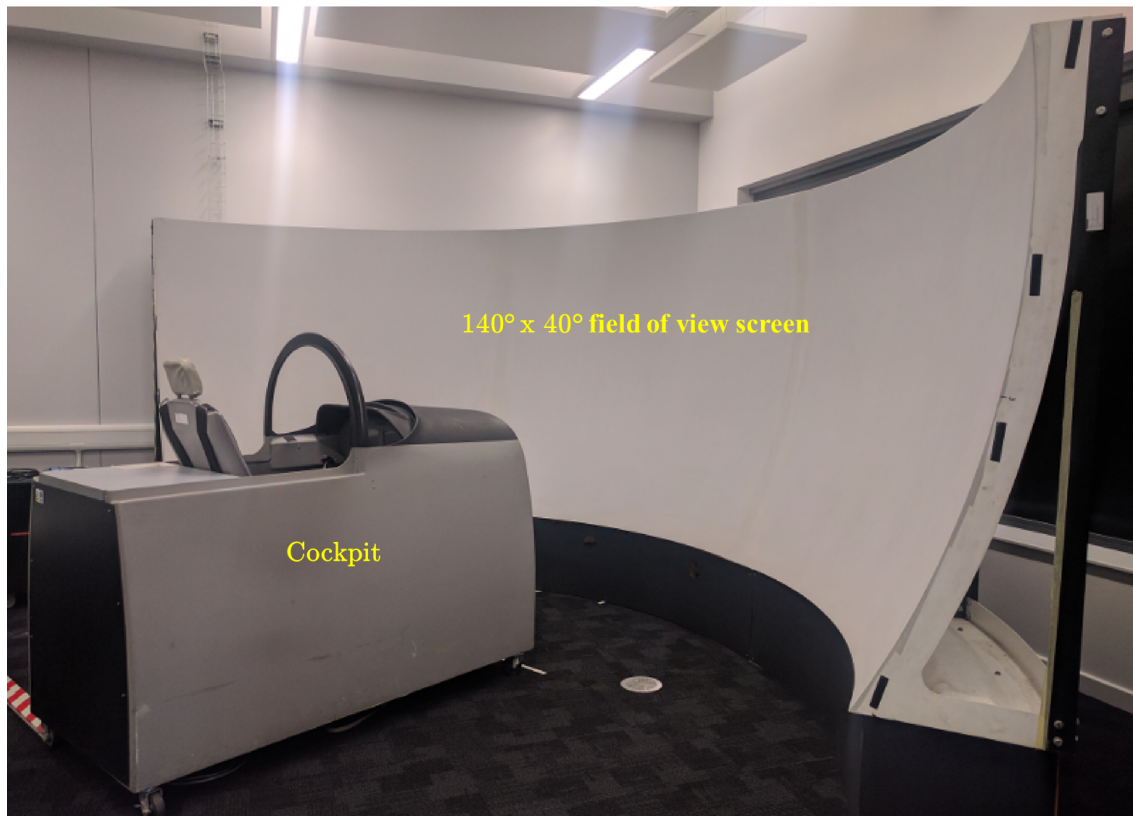
Figure 4.13: Overall setup of the EFS500 flight simulator
