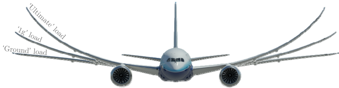
Figure 2.3: Wing deflection of Boeing 787 aircraft under ground, 1g and ultimate loading (reproduced from Ref. [23])
