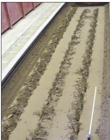
Figure 4.1-3 A completed soil-bin 'run' at 100 mm depth and 10^\circ vertical at 10^\circ horizontal (left), -5^\circ horizontal (middle), and 5^\circ horizontal (right).
