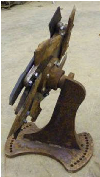
Figure 3.1-4 Independently mounted soil aerator bladed disc and arm unit
