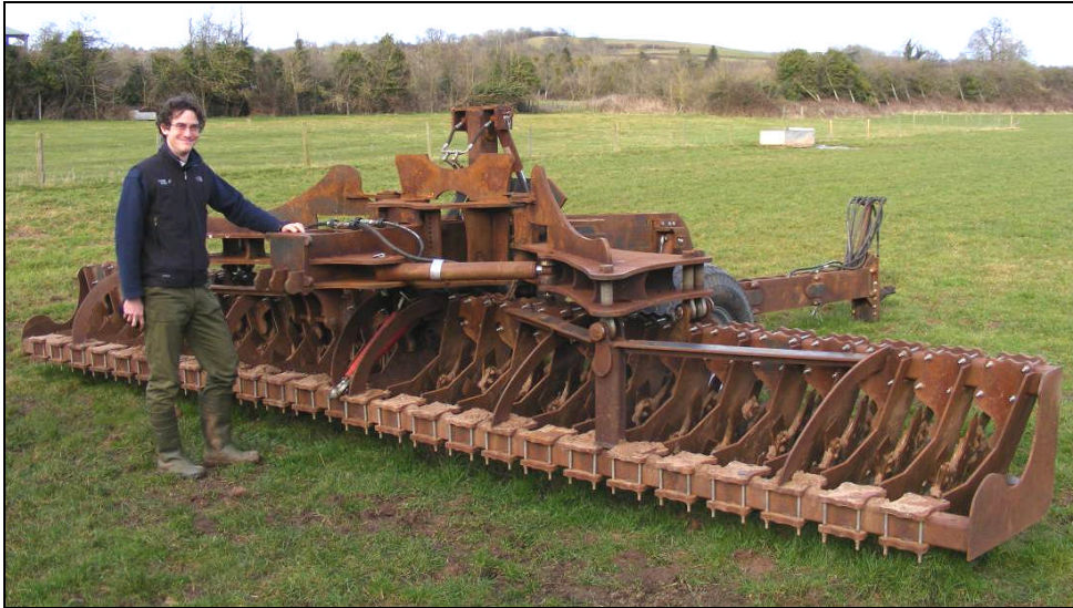
Figure 3.1-3 The 6.8 m wide soil aerator unit with two sets of twelve bladed discs
