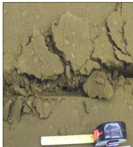
Figure 4.1-4 Soil breakout through soil aerator blade engagement at 100 mm depth, 18^\circ vertical and 0^\circ horizontal (note lifting and displacement of soil surface, tape at 100 mm)
