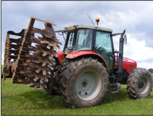
Figure 3.3-3 Soil aerator linkage-mounted to a Massey Ferguson 6480
