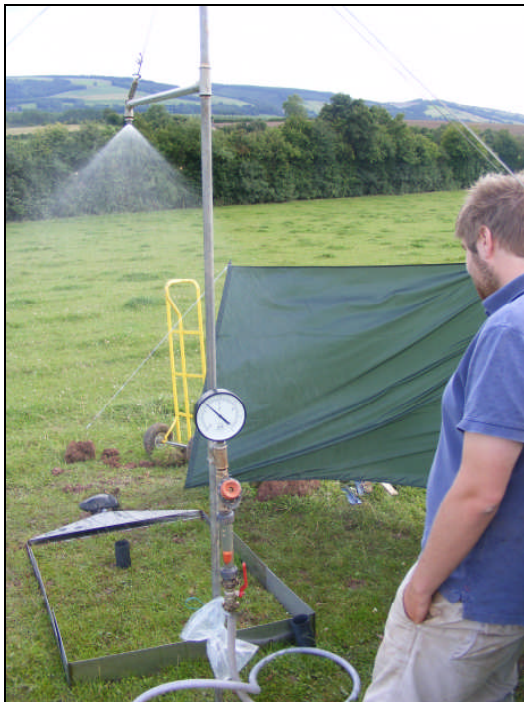
Figure 3.3-5 Complete setup of rainfall simulator (note the pressure gauge and regulating valve below gauge dial, uniform spray from nozzle and wind-break)
