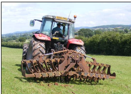
Figure 3.1-2 Linkage-mounted soil aerator with two sets of six bladed discs
