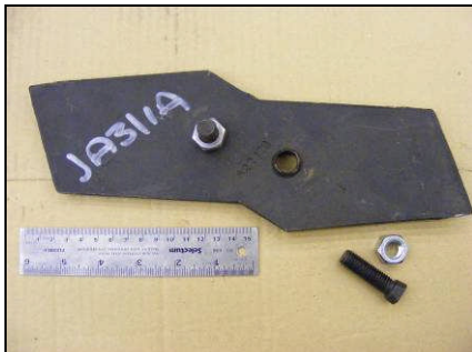
Figure 3.1-1 Soil aerator blade and attachment bolts (rule 150 mm in length)
