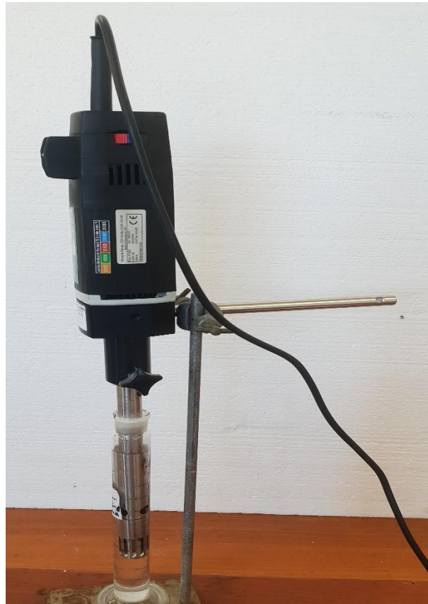
Figure 5.1 , X 620 high shear mixer used for water dispersion+
