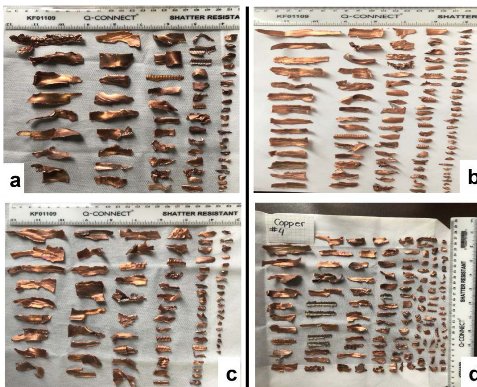
Figure 2. Photographs of the front face of strawboards, a) copper, end, b) copper mid, c) brass, end, d) brass mid
