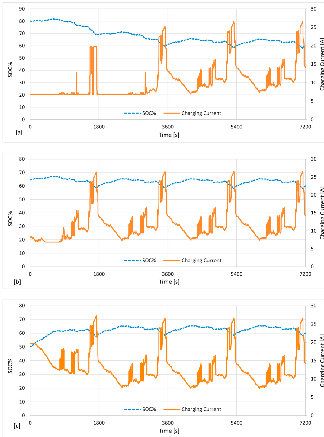
Fig. 11. Battery SOC and FC current graphs during the WLTP simulation for different initial SOC: a) 80%, b) 65%, and c) 50%.
