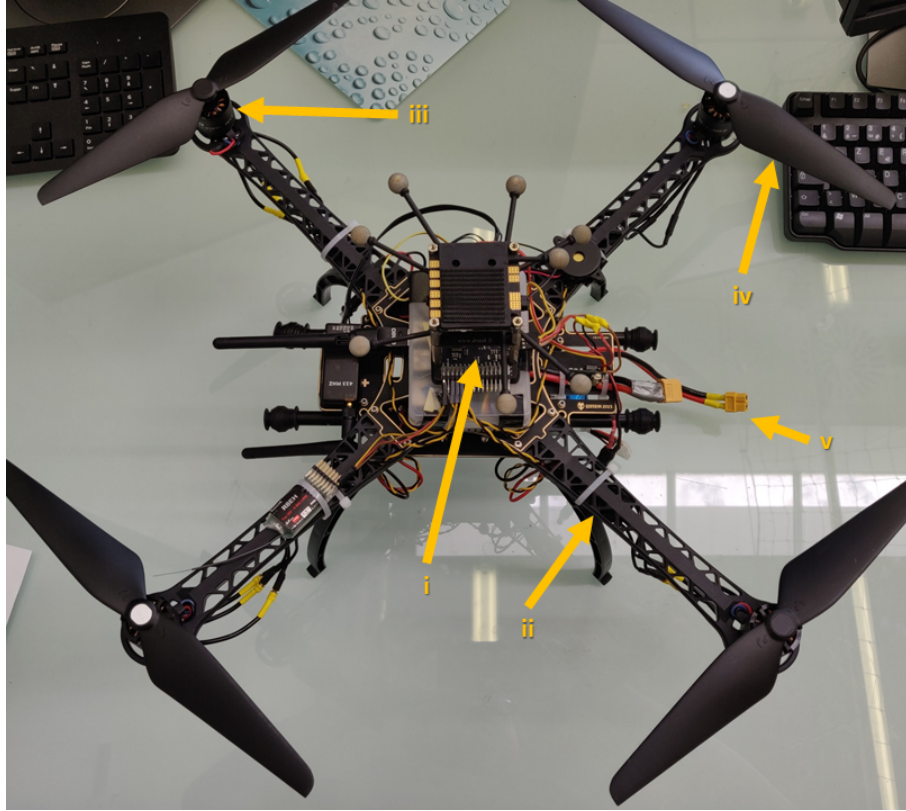
Figure 3.1: Multirotor in quad X configuration with visible components of the propulsion chain. (i) Flight Controller, (ii) ESC (under arm), (iii) BLDC Motor, (iv) propeller, (v) battery connector.
