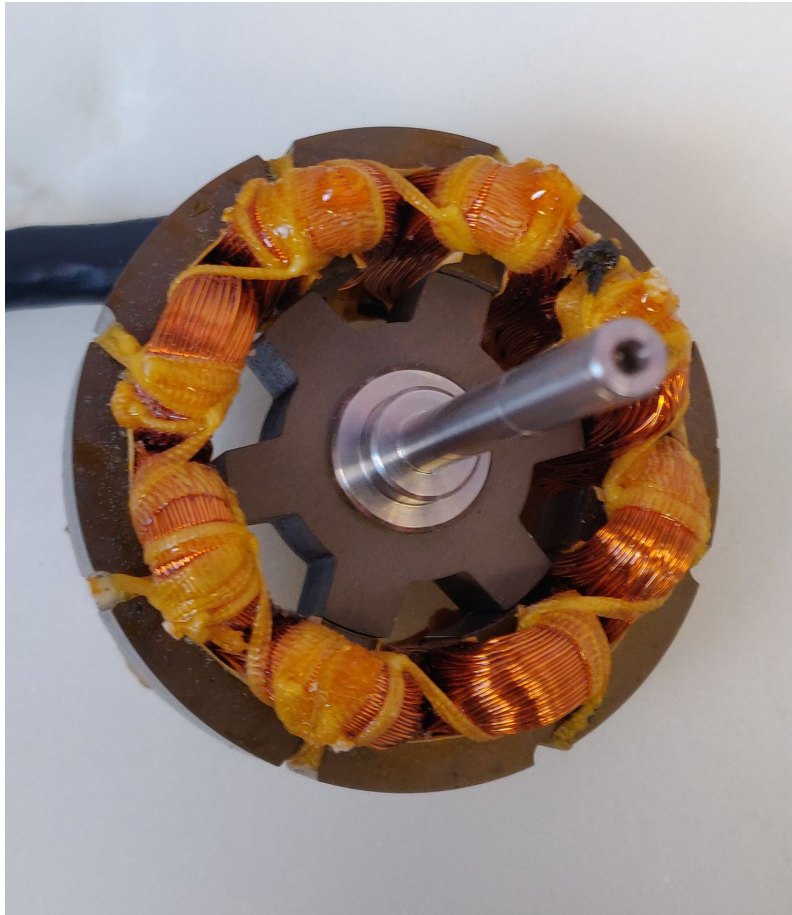
Figure 5.18: Manufactured 71x15-30 SR motor with shaft.
