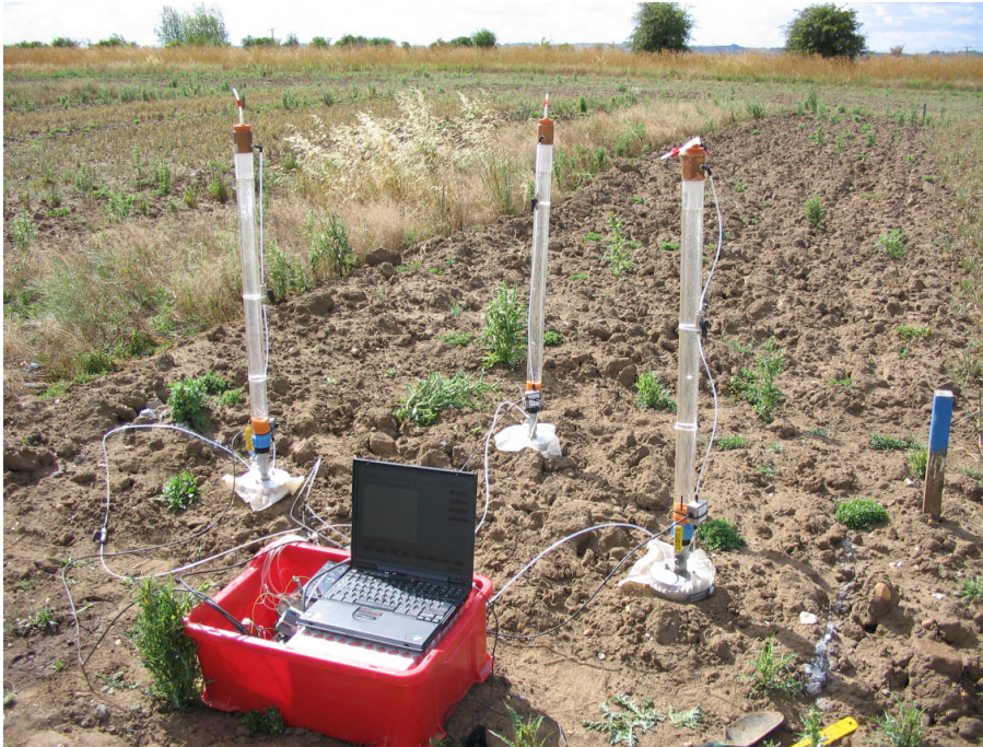
Figure 28. Experimental set up of the automated tension infiltrometer on a sandy loam soil.
