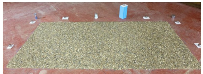
FIGURE 6 Image showing the gravel rectangle, together with spheres and top hat scatterers used to ensure image alignment.
