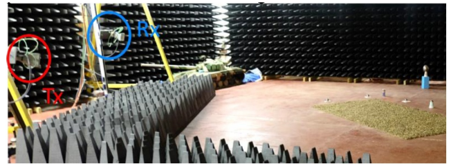
FIGURE 5 The Ground Based Synthetic Aperture Radar (GBSAR) laboratory in a bistatic configuration. The transmitter is circled in red and labelled Tx; the receiver is circled in blue and labelled Rx.
