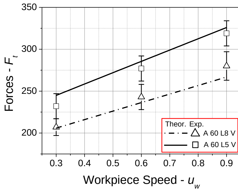
Figure10. Comparison between experimental measurements and theoretical predictions for grinding wheels with different structure grades
