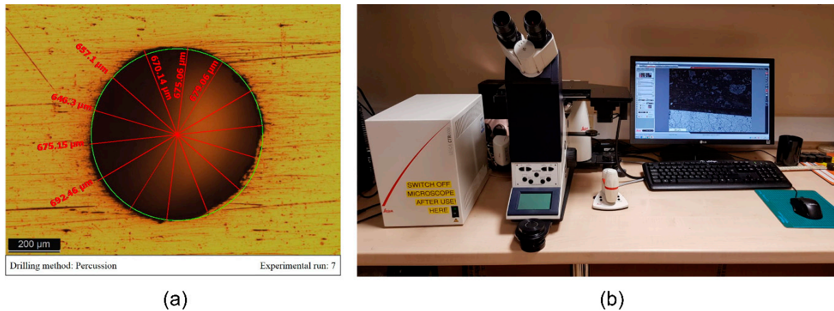
Figure 5. (a) Strategy for measuring hole diameter. (b) Leica optical microscope.
