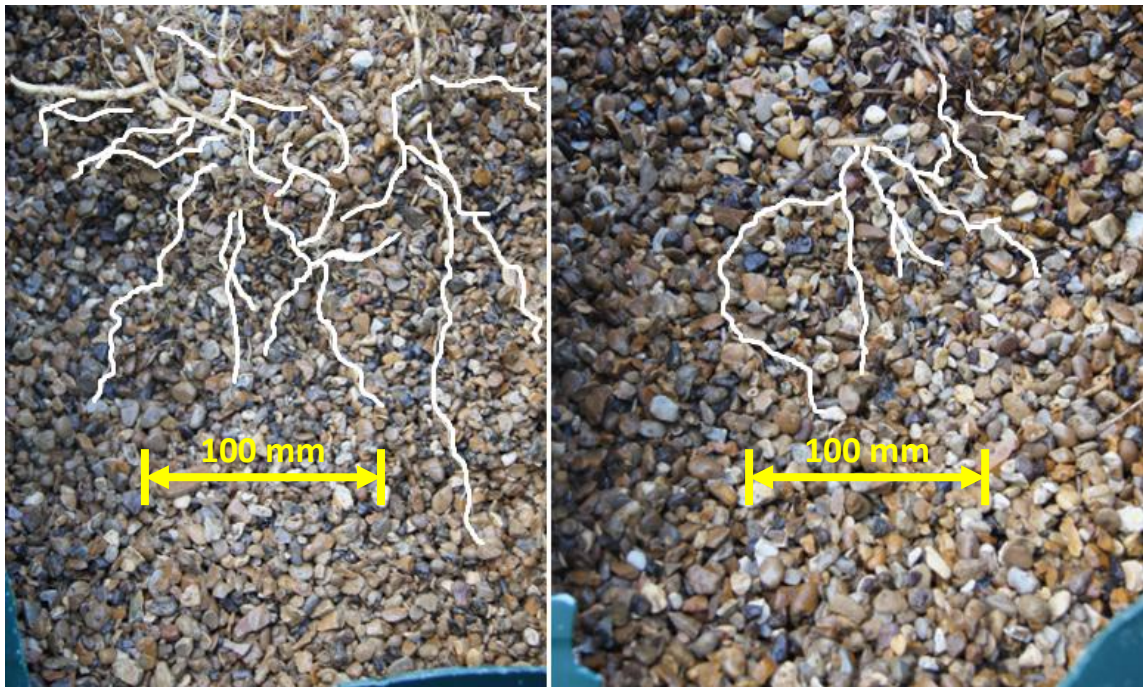
Figure 6 Example of root systems in-situ (enhanced): (a) P. australis control and (b) P. australis high aeration.
