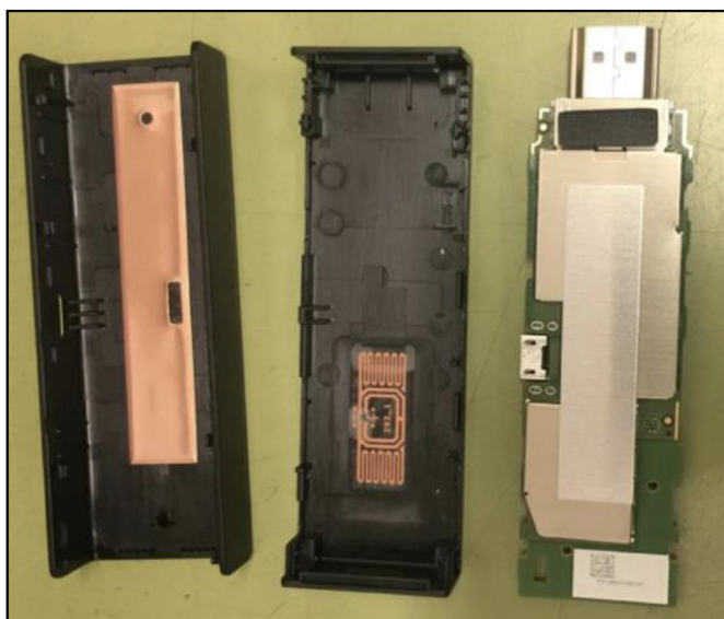
Fig. 2. Amazon firestick with outer casings removed.
