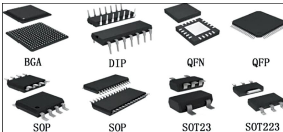
Fig. 4. Integrated circuit package types (Electronicsforu, 2019).
