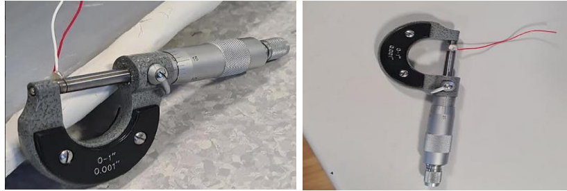
Figure 3-25 Measured dimensions of the PZT using a micrometre screw gauge.
