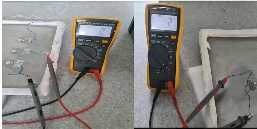
Figure 3-26 The measured capacitance of the installed exciter and sensors using a Fluke digital multimeter.
