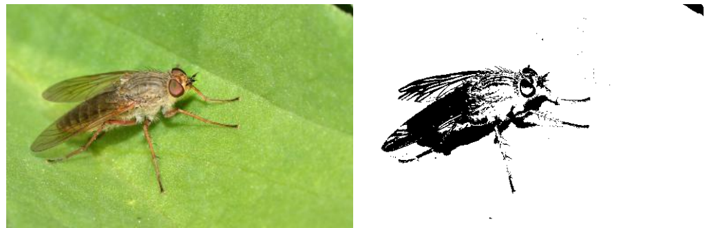
Figure 6. Demonstration of image binarisation for segmentation: (Left) original input image, (Right) binary image resulting from threshold-based segmentation.
