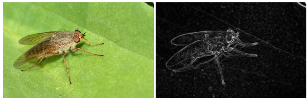
Figure 5. Demonstration of the Sobel edge detection operator: (Left) original input image, (Right) resulting image after edge detection.
